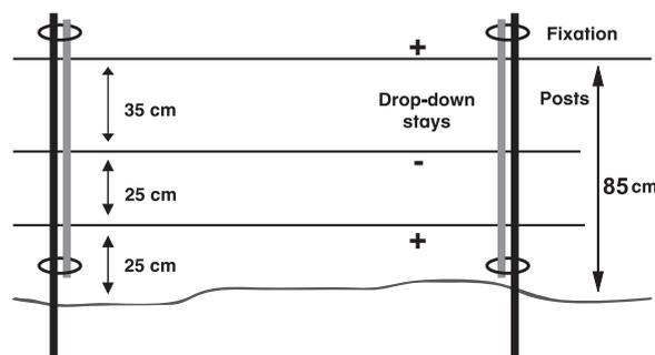
**Fig. 2.** Design proposal of a guanaco friendly high tensile electric fence for livestock in arid Patagonia. Hot and ground wires are attached to drop-down stays that are fixed to posts. Top wire height is lower than current ovine design and larger space between wires would allow crossing of yearling and reduce entanglement.
